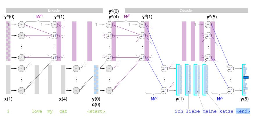
The sequence-to-sequence RNN directly calculates  $p(y \mid x)$ :
